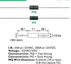
MS Wire Diameter: 0.81 mm (All ratings) Sample P/N: MQ002 for a 2A fuse.
