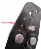
Step 4. Crimp terminal to wire. Repeat for each of the 4 cables.
