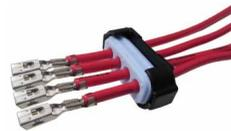
All terminals now crimped onto cables.
