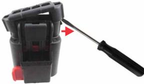
Step 1. Gently pry the cable cover off using a small flat head screw driver.
