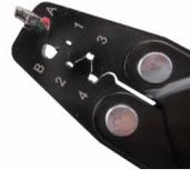
Step 5. Crimp terminal to insulation. Repeat for each of the 4 cables.
