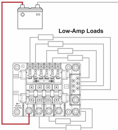
Battery power is connected to one of the 4 MIDI fuses to supply power to all fuse circuits. This Midi fuse acts as a main fuse to protect against total current draw in excess of 170A (assuming a 200A Midi fuse is fitted). If you wish to operate higher current, please refer to P/N: 880089 which is rated to 600A max using a power input stud instead of a Midi fuse.
